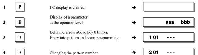
The seam functions (e.g. sewing foot lift, start backtack, etc.) can be programmed using the keys on the control panel.
