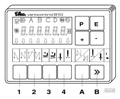
The V810 control panel is supplied with slide-in strip **no. 1** above the keys. For different functions the strip can be replaced with a different one supplied with the control panel. Set parameter **291** in this case. See also **V810** / **V820** instruction manual!
