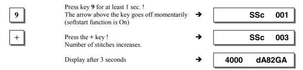
This value is saved when you start sewing. It remains in effect even after turning the machine off!
