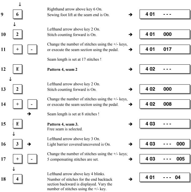
If a different key is pressed, end backtack section input is completed, and the lefthand arrow above key 4 stops blinking. The single end backtack is enabled.
