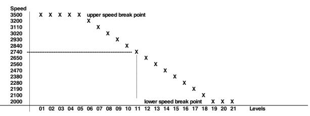
Display example of parameter 182 on the V820 control panel:
