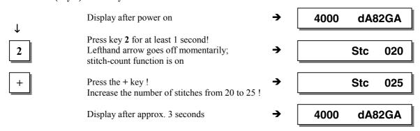
This value is saved when you start sewing. It remains in effect even after turning the machine off!
