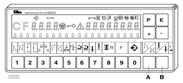
The V820 control panel is supplied with slide-in strip **no. 1** above the keys.
