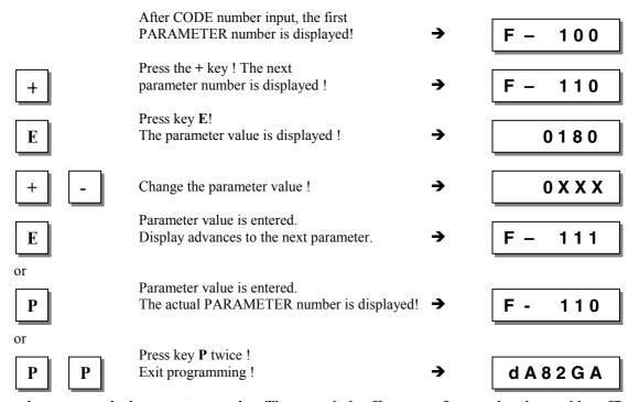
These values are saved when you start sewing. They remain in effect even after turning the machine off!
